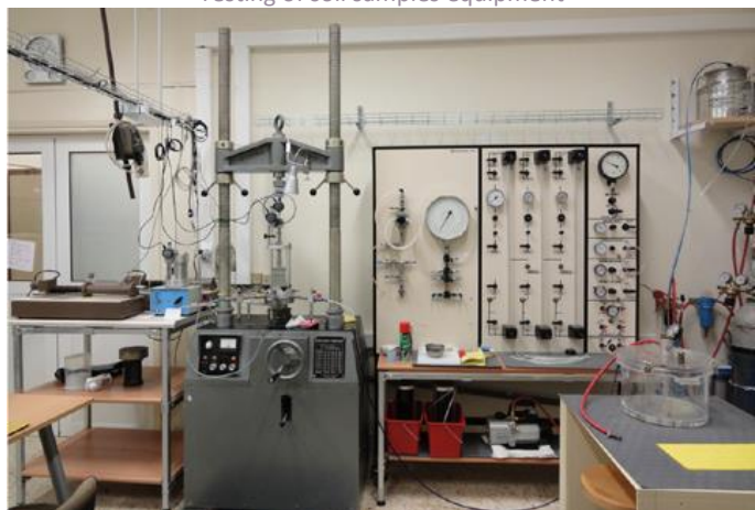
Triaxial device – SoilTest 25Tons
