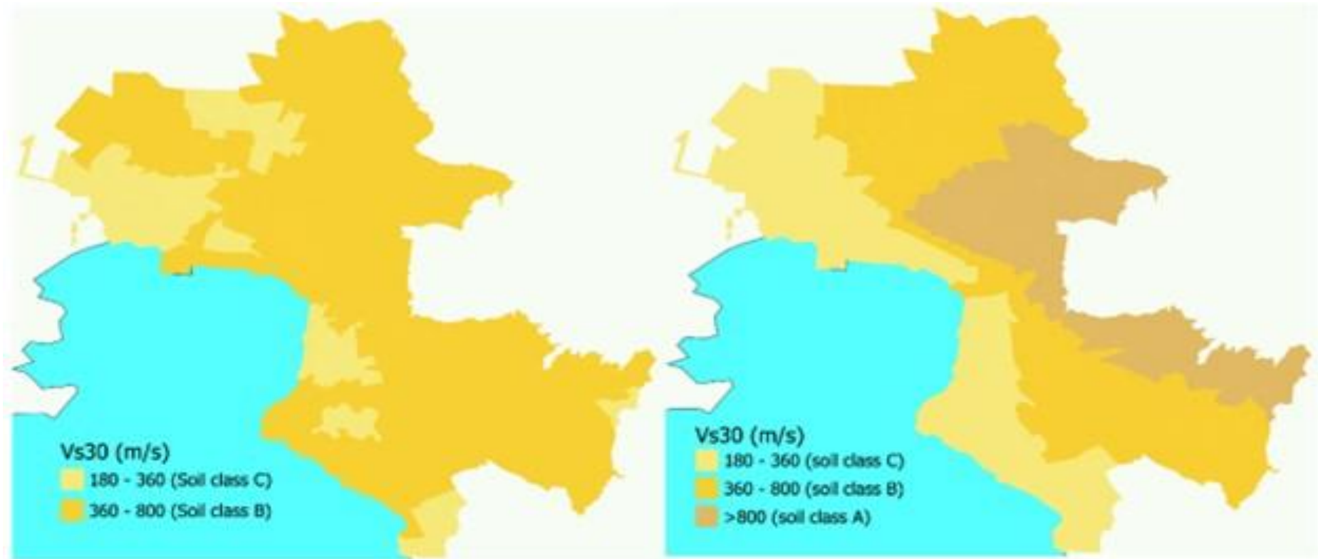
Spatial distribution of Vs.30 models of Thessaloniki according to USGS slope-based model (left) and measured values (right)
