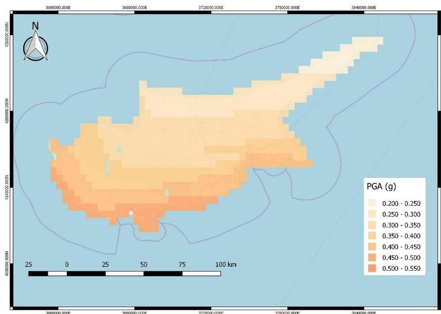
**Figure 14** – Mean seismic Hazard map in PGA for probability of exceedance 10% in 50 years (T=475 years)
