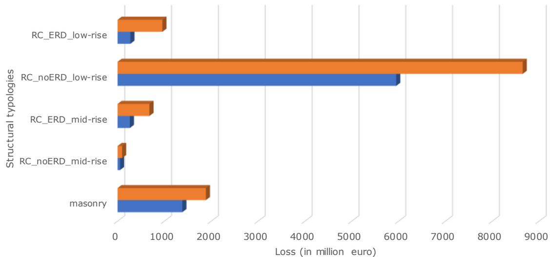
**Figure 31** – Loss per structural typology with 10% and 2% probability of exceedance in 50 years (T=475 and 2500 years)
