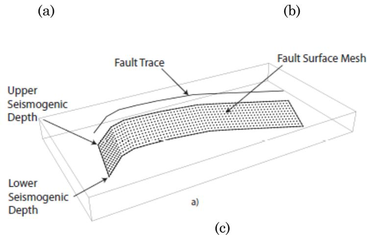
**Figure 8** – Graphical representation of earthquake ruptures (a) as generated by point sources for different input parameters ; (b) as generated by an area source, mainly originated by point sources uniformly distributed along an area ; (c) as a portion of a fault surface mesh, simulated in OpenQuake engine (Pagani et al., 2014)
