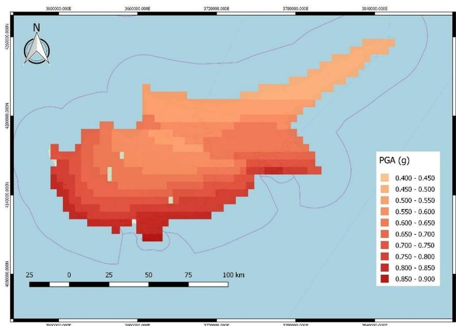
**Figure 15** – Mean seismic Hazard map in PGA for probability of exceedance 2% in 50 years (T=2500 years)
