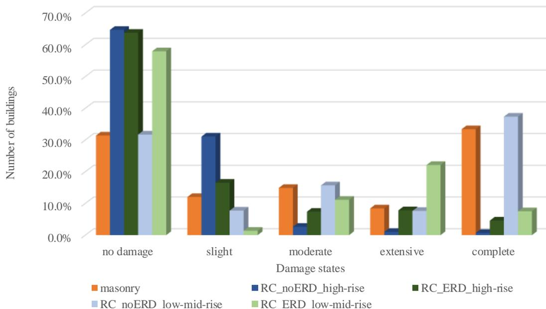
**Figure 42** – Disaggregation of ratio of damaged buildings per damaged state and structural typology for seismic scenario with T=475 years
