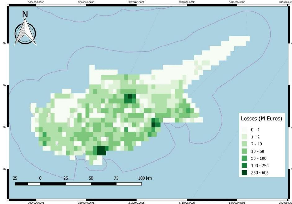
**Figure 34** – Loss map (in million euro) for seismic scenario with 10% probability of occurrence in 50 years ( $T=475$  years)
