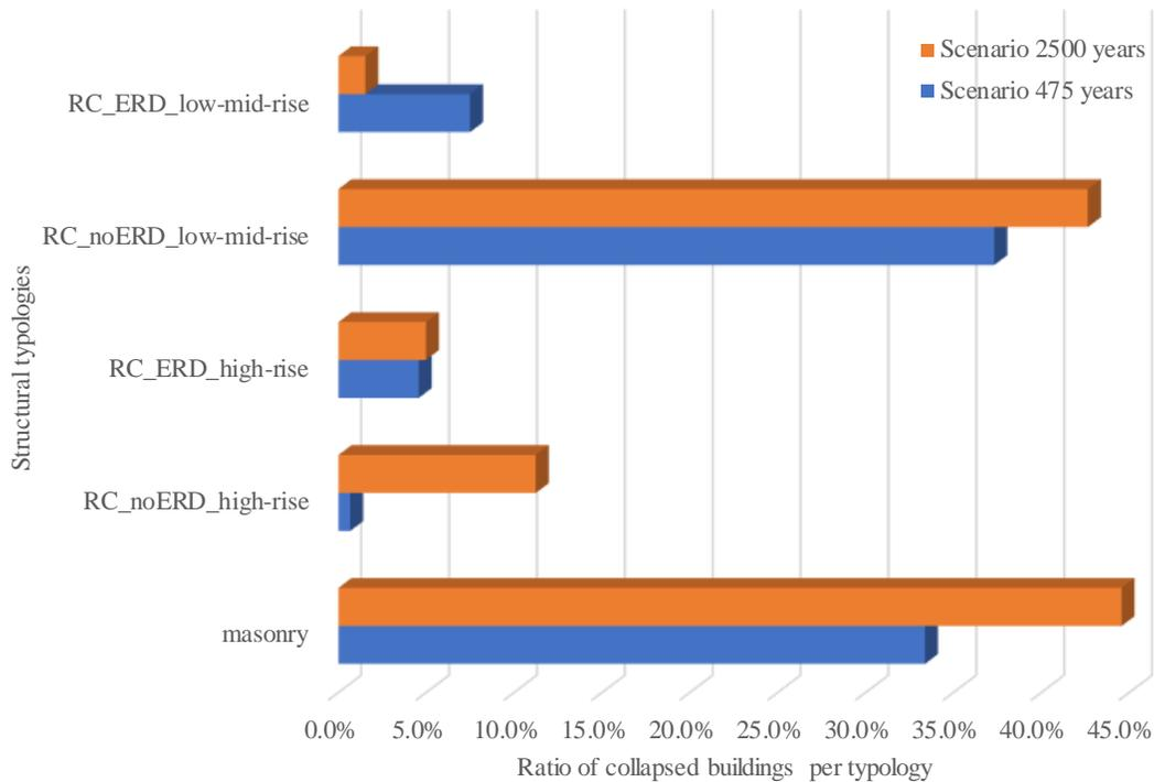
**Figure 41** – Ratio of collapsed buildings over total number of buildings per typology for the two studied scenarios
