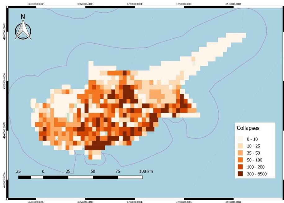
**Figure 35** – Collapse map (in number of buildings) as a result of damage assessment for a seismic scenario with 10% probability of occurrence in 50 years ( $T=475$  years)
