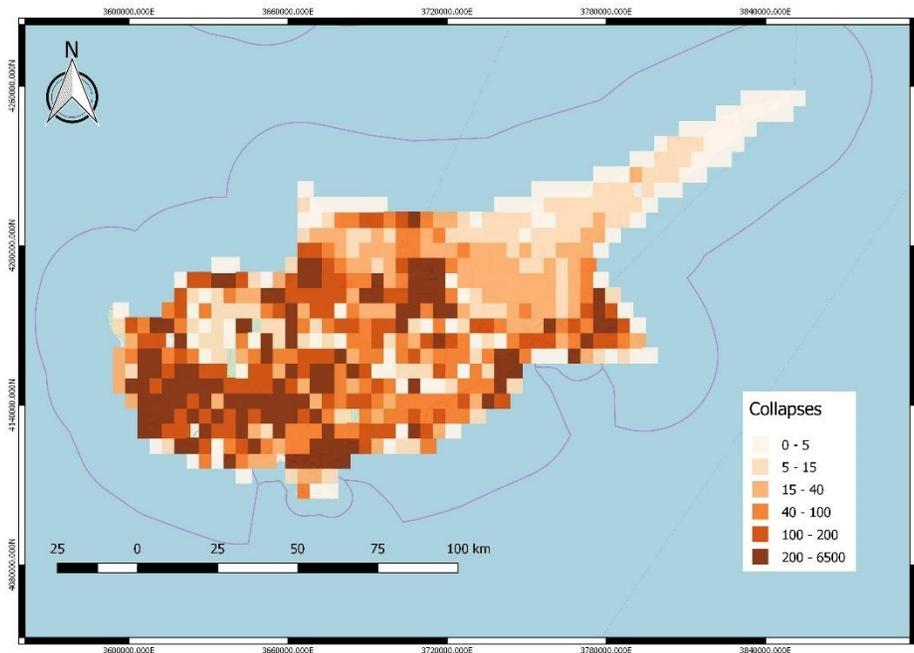
**Figure 37** – Collapse map (in number of buildings) as a result of damage assessment for a seismic scenario with 2% probability of occurrence in 50 years ( $T=2500$  years)
