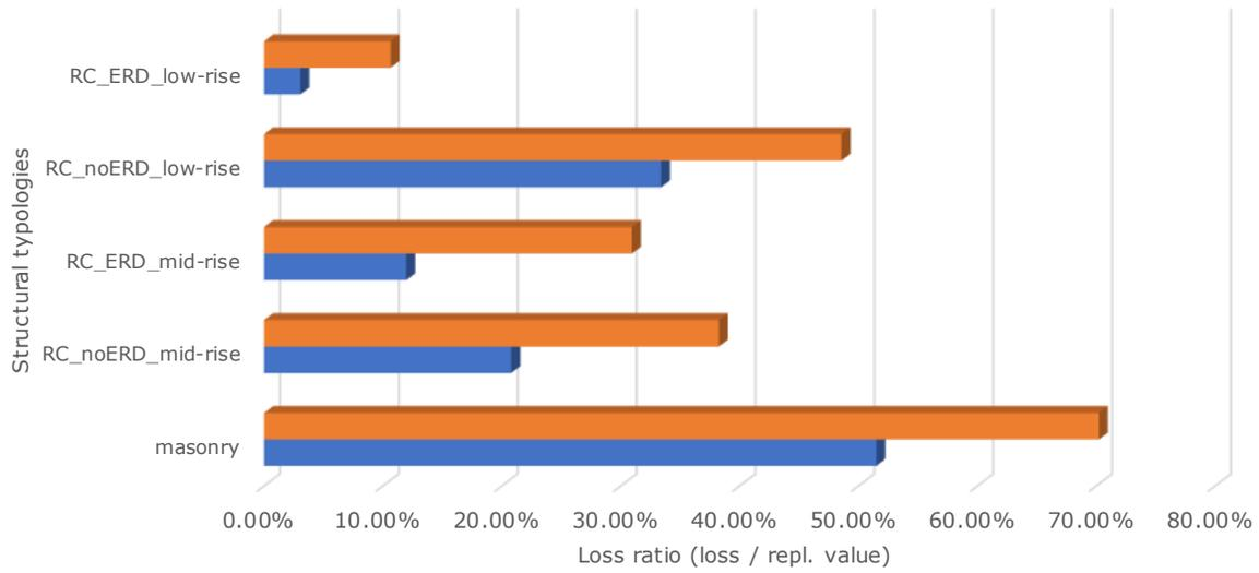
**Figure 32 – Loss ratio per structural typology with 10% and 2% probability of exceedance in 50 years (T=475 and 2500 years)**
