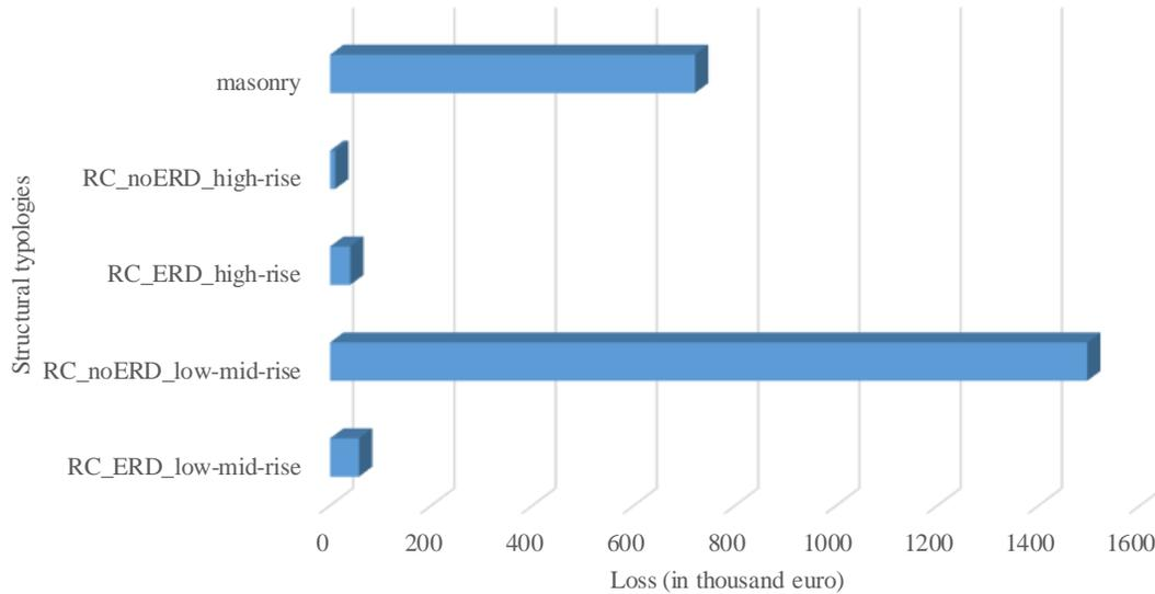
**Figure 27 – Disaggregation of average annual loss per structural typology**
