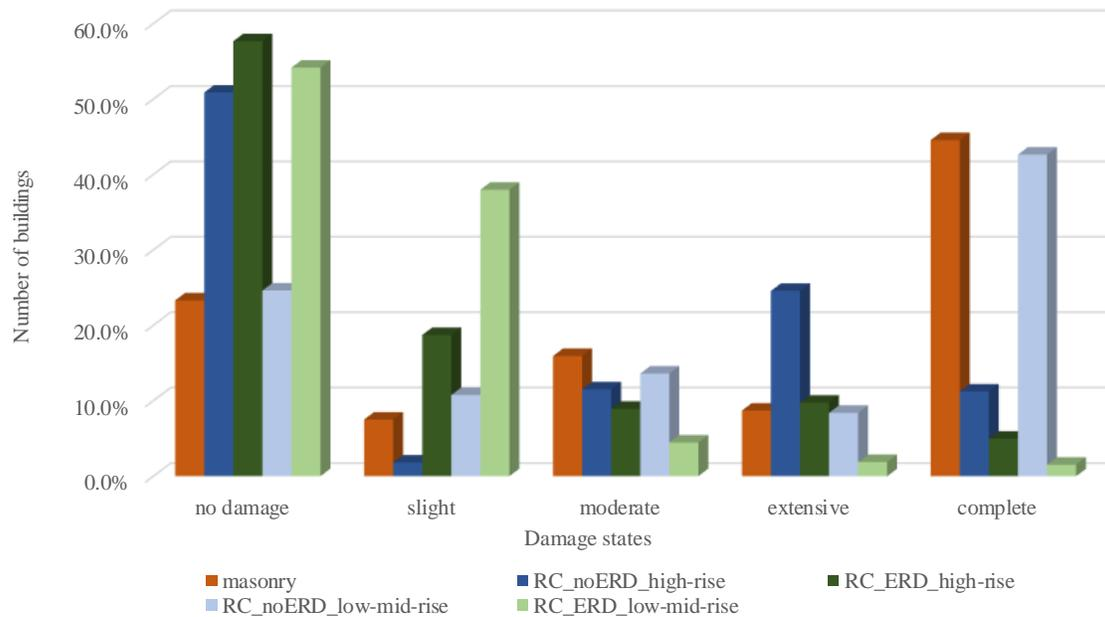
**Figure 43** – Disaggregation of ratio of damaged buildings per damaged state and structural typology for seismic scenario with T=2500 years
