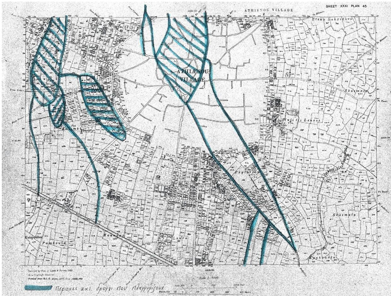
**Figure 54 – Vulnerable to flooding areas (blue highlight)**
