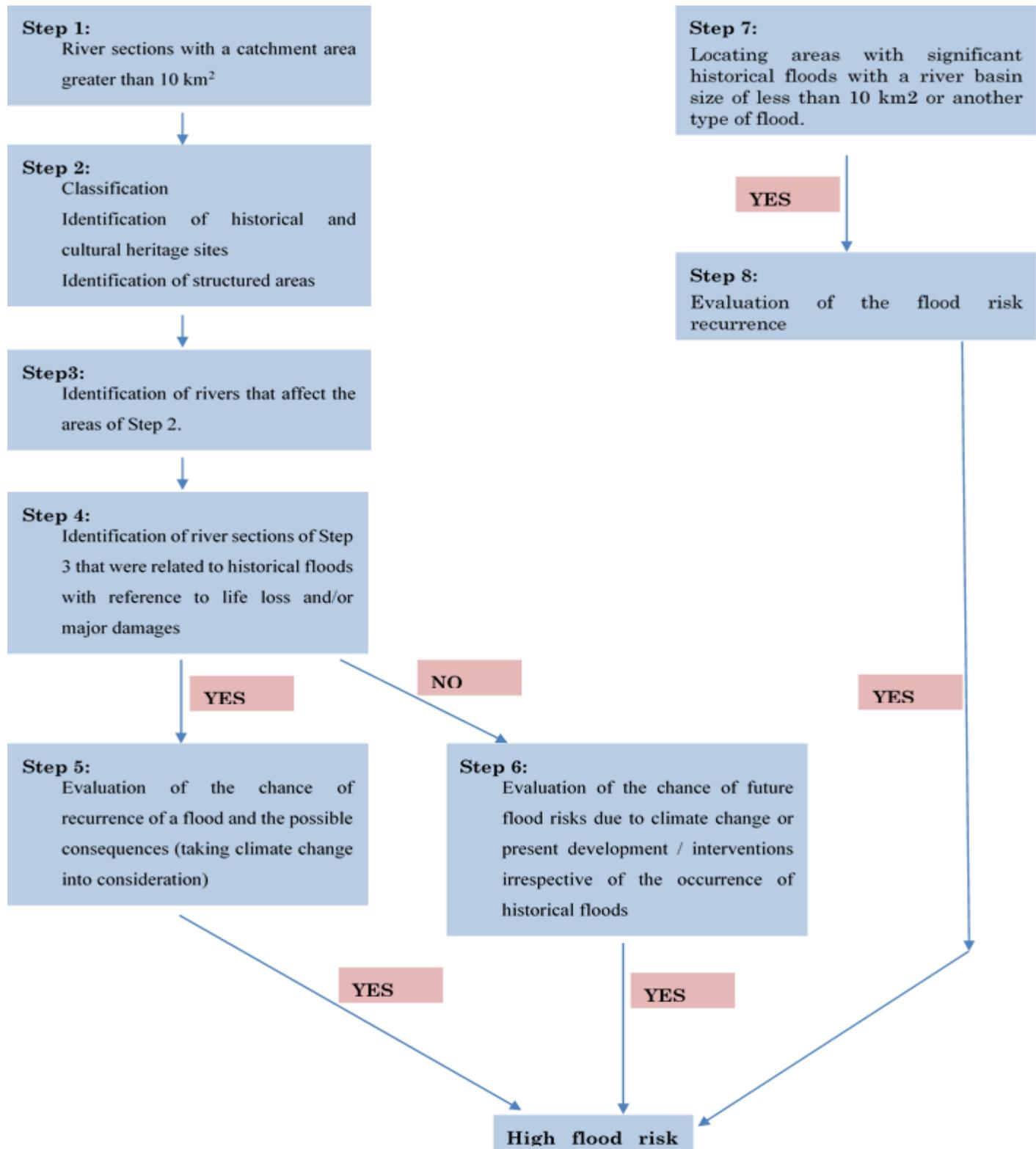
Figure 50 – Methodology for identifying areas with significant potential flood risks
