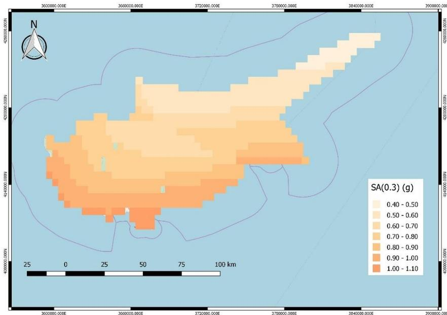
**Figure 16** – Mean seismic Hazard map in Spectral acceleration at  $T=0.3$  s for probability of exceedance 10% in 50 years ( $T=475$  years)
