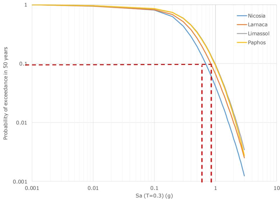
**Figure 13** – Hazard curves for the main cities of Cyprus in Spectral acceleration at T=0.3 s from PSHA
