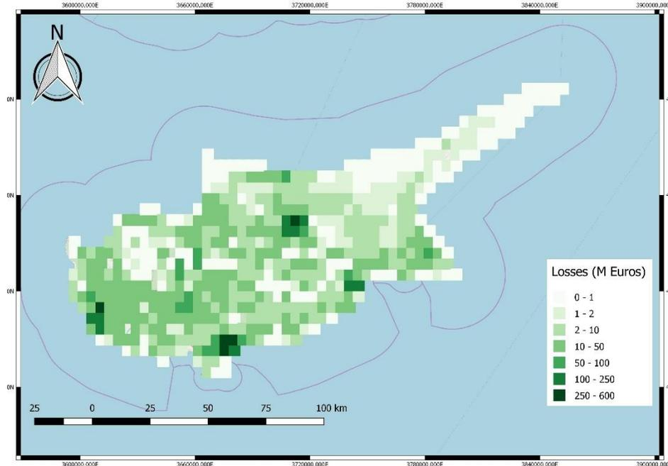
**Figure 36** – Loss map (in million euro) for seismic scenario with 2% probability of occurrence in 50 years ( $T=2500$  years)
