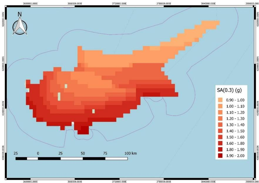
**Figure 17** – Mean seismic Hazard map in Spectral acceleration at  $T=0.3$  s for probability of exceedance 2% in 50 years ( $T=2500$  years)
