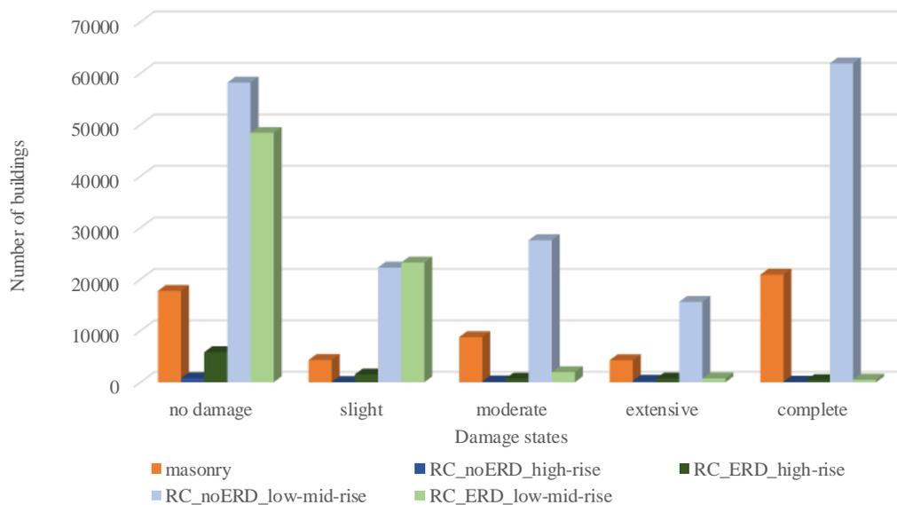
**Figure 39** – Disaggregation of damaged buildings per damage state and structural typology for seismic scenario with T=475 years
