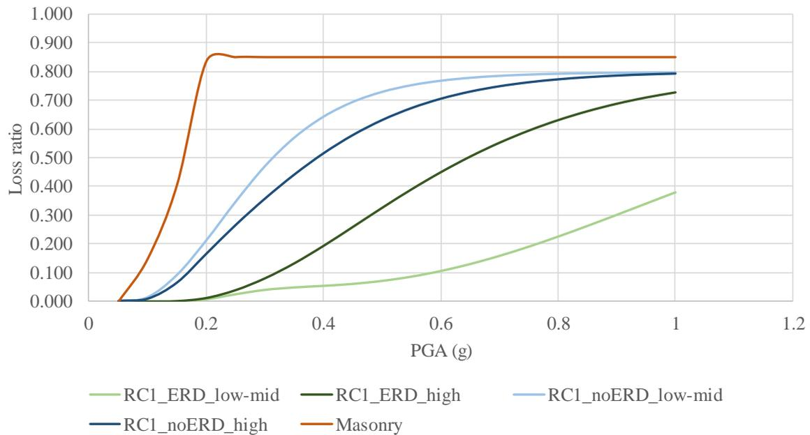
**Figure 25 – Loss functions for all structural typologies**
