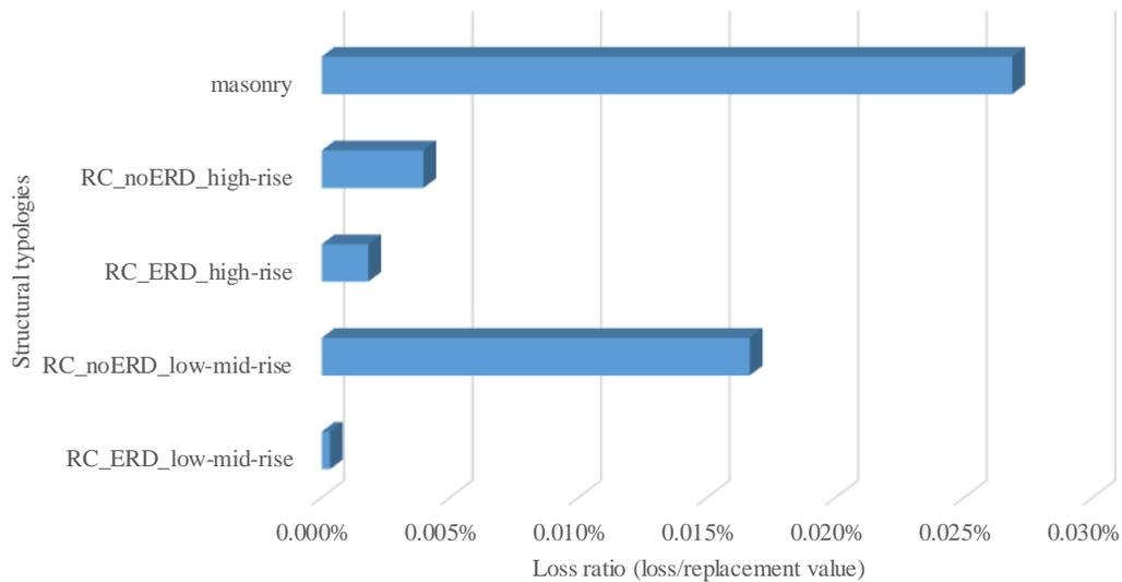
**Figure 28 – Disaggregation of average annual loss ratio per structural typology**
