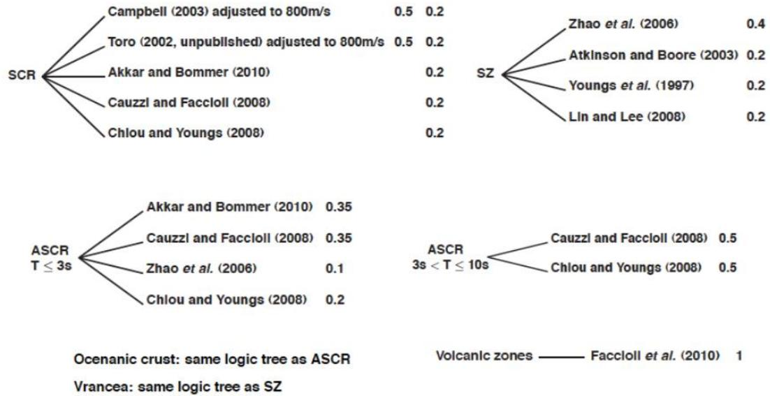
Figure 10 – Ground motion prediction equation logic tree for SHARE (Woessner et al., 2013)
