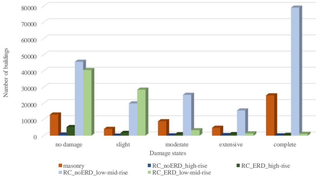
**Figure 40** – Disaggregation of damaged buildings per damage state and structural typology for seismic scenario with T=2500 years
